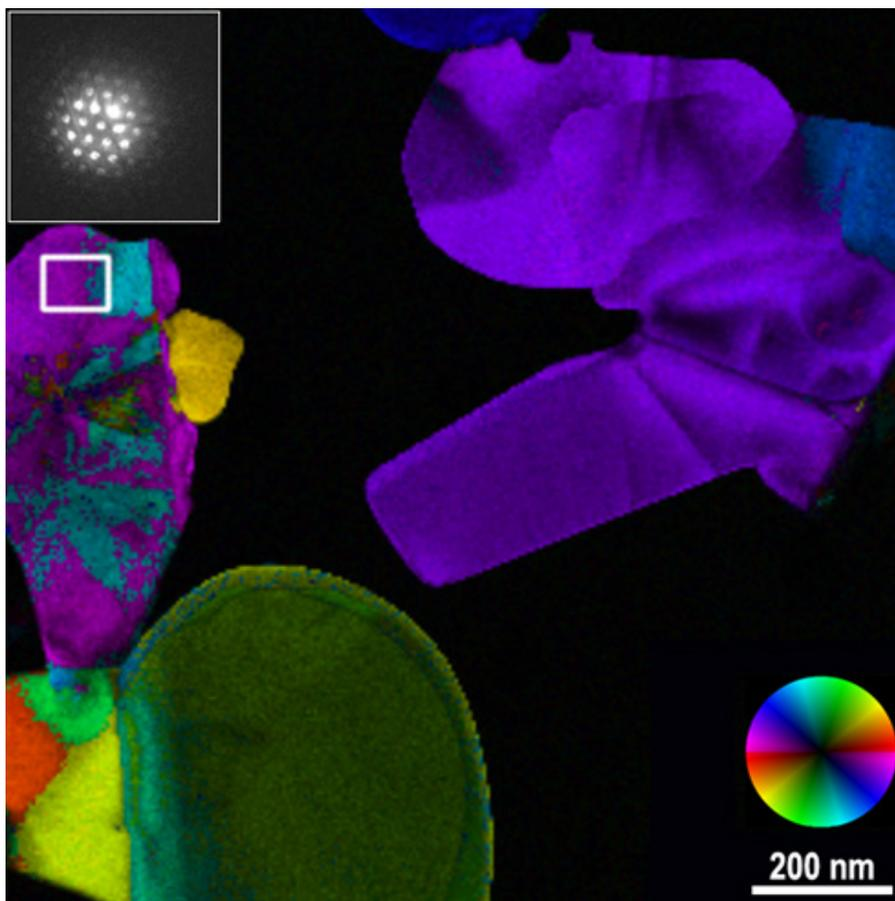
**Figure 1.** Map of boron nitride from a counted 4D STEM dataset collected with the Metro camera. A color scale is shown at the bottom right, to indicate which color corresponds to each angle, as well as the brightness variation from very dim spots (center) to very intense spots (edge). The inset shows the sum of diffraction patterns from the region in the white rectangle.
